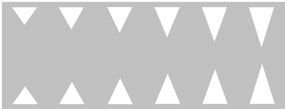
Figure 17 : Dragon's Teeth Road Markings
