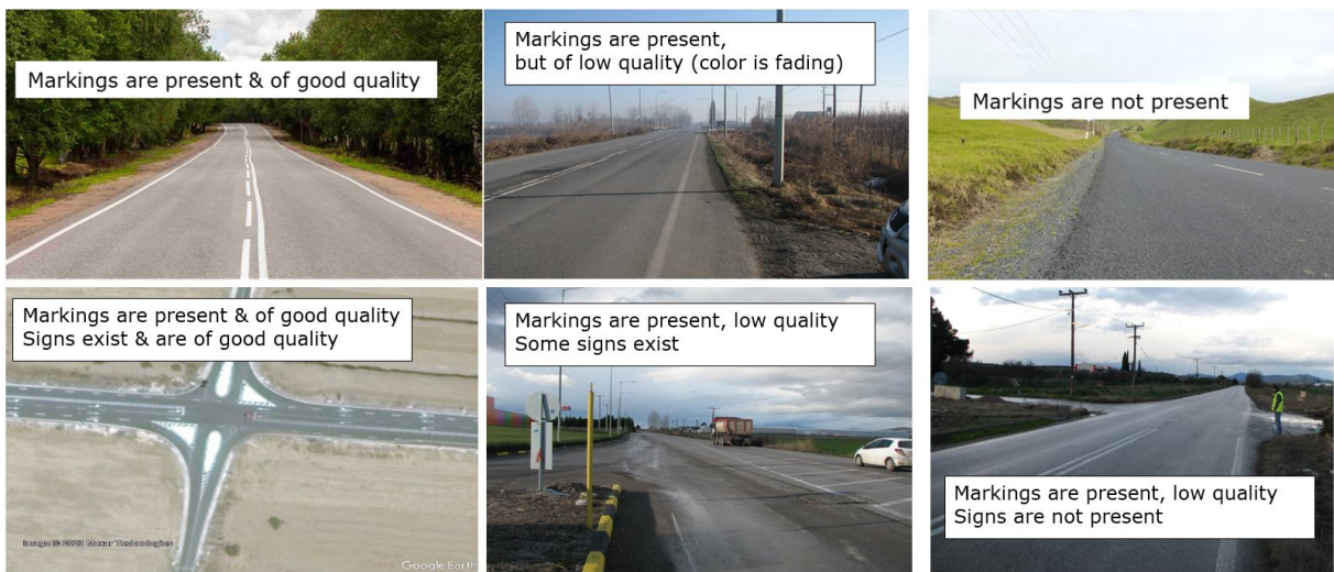
Figure 3.22: Example of segments and intersections where markings and signs are present, of good or low quality or not present
