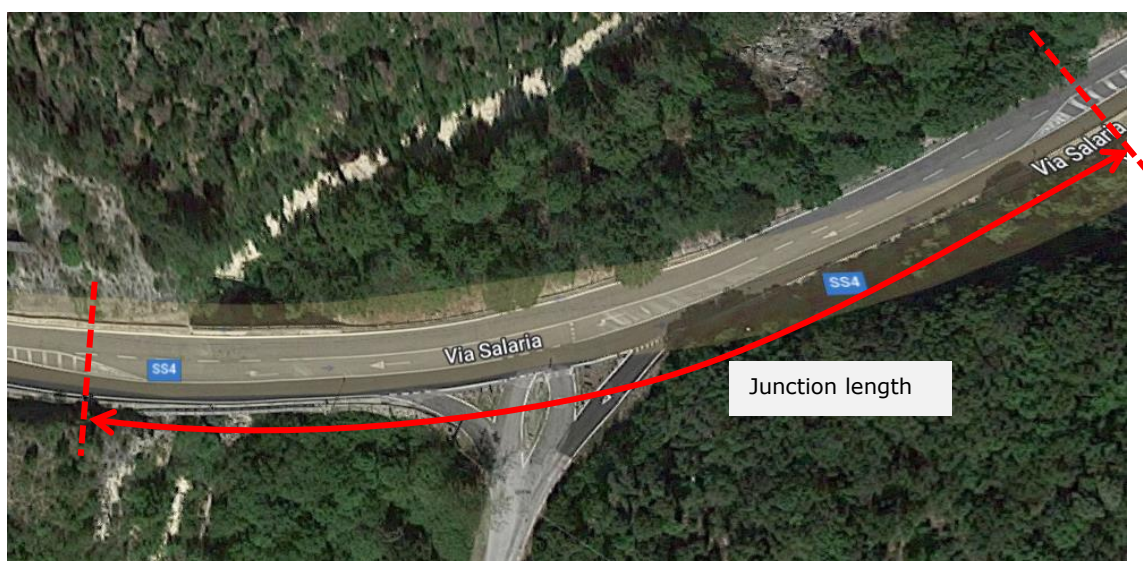
Figure 2.2: Example of segmentation at the area of an at-grade intersection.
