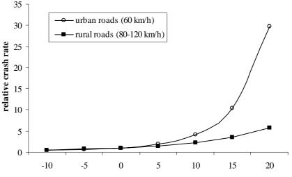
vehicle speed in relation to average traffic speed (in km/h)
