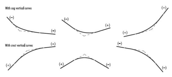
Figure 5 Examples of vertical alignment (PIARC 2003)
