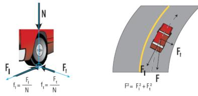
Figure 9 Longitudinal and transverse friction
