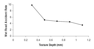
Figure 10 Relationship between Wet-Accident and Surface Texture Depth (Gothie 1991)
