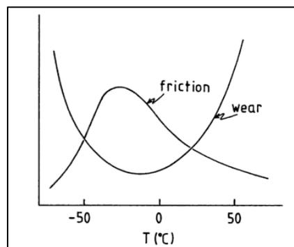
Figure 4: Relation of friction and wear versus temperature of a rubber compound [4].
