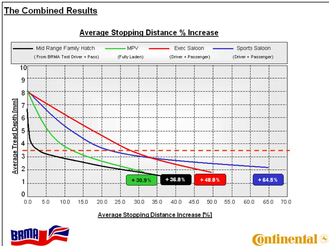
Figure 7: Percentage change in stopping distance versus tread depth [6].
