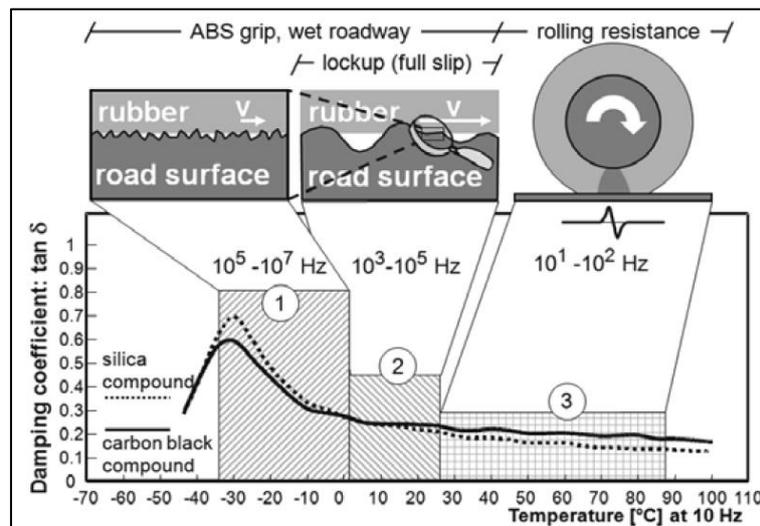
Figure 3: Energy loss versus temperature curve showing the excitation frequencies experienced by a tyre [3].
