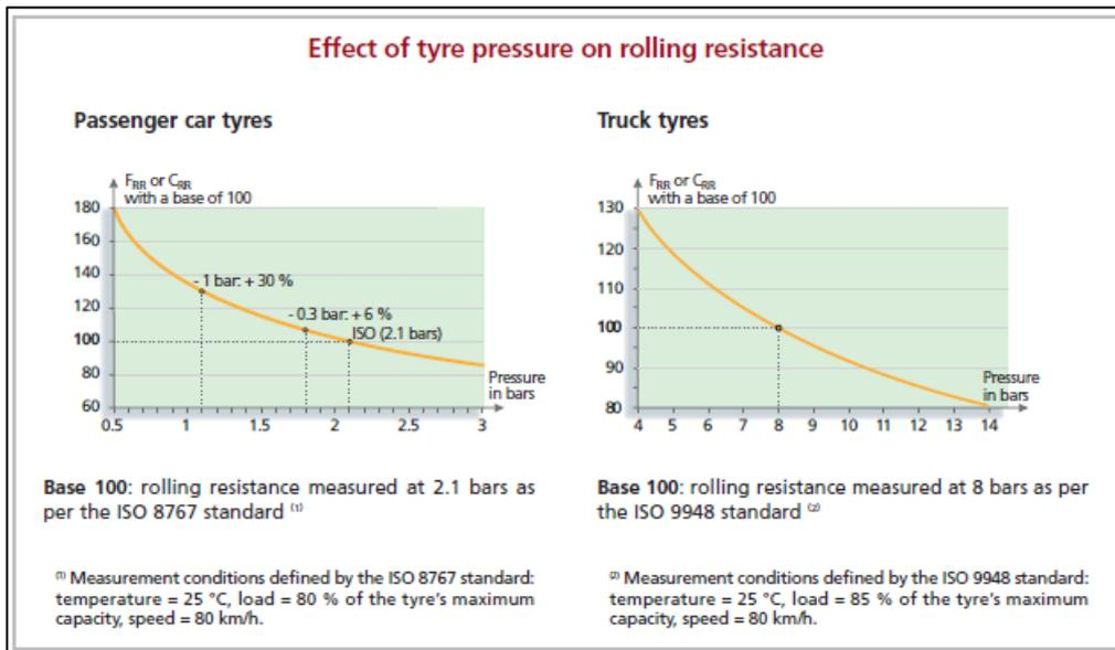
Figure 10: Effect of tyre inflation pressure on rolling resistance [8].
