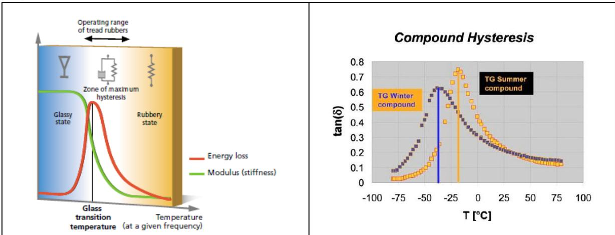
Figure 2: Left graph showing energy loss ( $\tan(\delta)$ ) [2] and right graph shows modulus of tread rubber compounds [1].
