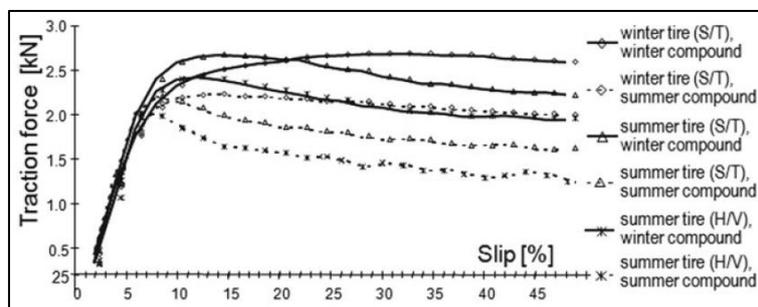
Figure 5: Curves showing the effects of tyre type and rubber compound on the coefficient of friction (snowy surface) [3].
