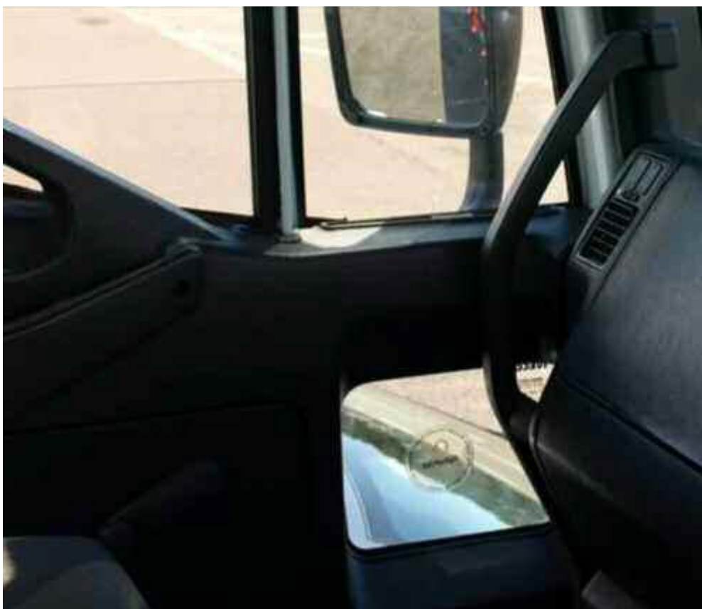
Figure 33: Example of side door designed to offer improved direct field of view, source (Dodd 2009)
