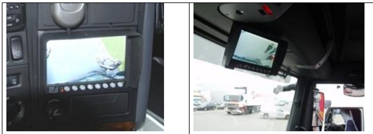
Figure 31: Examples of display positioning for camera systems, source www.orlaco.com
