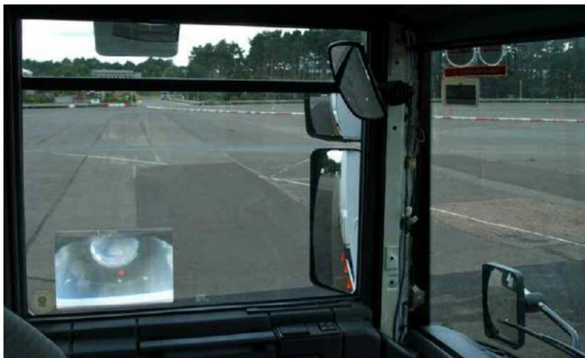
Figure 29: View from a Renault Magnum equipped with mandatory class II, IV and V mirrors plus Dobli and BDS mirrors and a frenal lens where a cyclist was positioned two metres ahead of driver's eyes at the edge of an adjacent lane.
