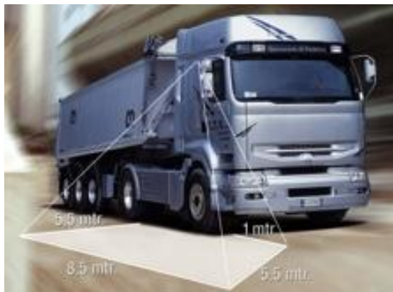
Figure 30: Example of field of view from a side view camera, source www.orlaco.com
