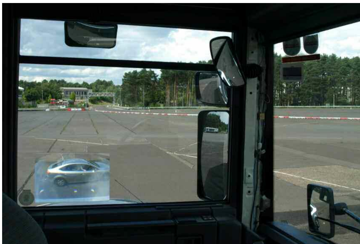
Figure 27: Vehicle equipped with mandatory mirrors and three supplementary field of view devices, source (Dodd 2009)
